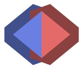
Figure 4-5: Demonstrating edge fattening and it's effects on capping. The brighter areas represent actual polygons from which the darker areas are calculated. Along contour lines, the fattened back-facing polygons will partially stick out from behind the front-facing polygons.
