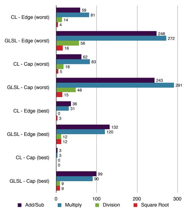
Figure 9-13: This chart shows the relative quantity of different types of mathematical operations used by both methods under different conditions. The author's method requires vastly fewer operations to its lack of duplication of work and test optimizations. Smaller is better.
