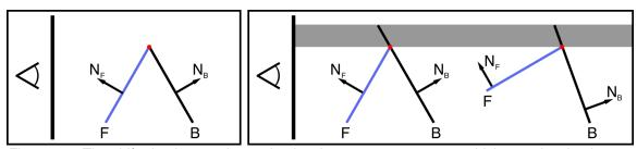
Figure 4-4: The shifted polygon edge maintains the same screen-space thickness despite the orientation of the polygons making up the edge.
