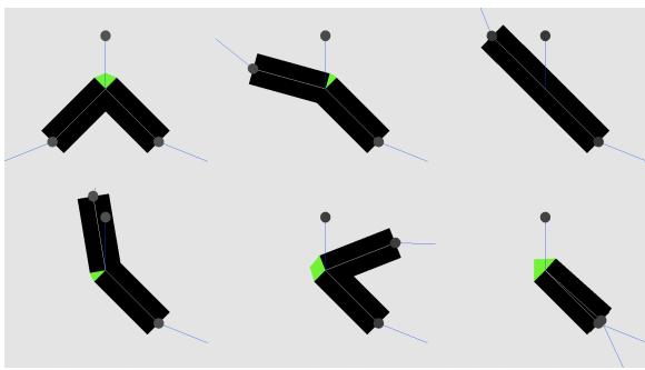
Figure 9-13: The green caps are generated without the use of the normal, and always perfectly fill the gap between the two edges because they are created utilizing the vertices of both edges.
