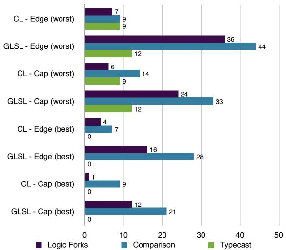
Figure 9-14: This is a comparison of the number of logic forks (if statements), comparison operations, and typecasts (vector types) used by each method under different conditions. The author's method does significantly fewer of these operations. Smaller is better.
