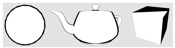
Figure 7-1: This variation uses a thresholding dot product check in a pixel shader. Some objects work better than others with this method, but the edge width is almost always inconsistent. The cube illustrates the main failure case for this method.
