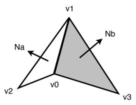
Figure 6-1: A single polygon edge connecting two adjacent polygons. Na and Nb are the face normals for the two adjacent polygons. v0 and v1 vertices define the edge. v2 and v3 complete the two adjacent polygon's vertices. The right polygon, and therefore the v3 vertex, may not exist. If so, the edge is a boundary edge.
