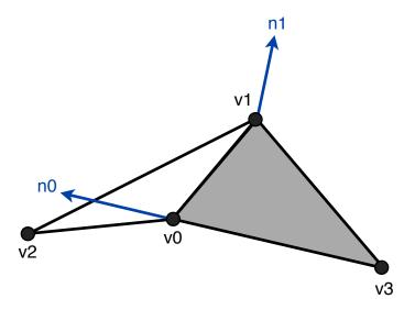
Figure 8-1: The important geometric values for each edge in McGuire and Hughes' method: v0, v1, v2, and v3 are vertices on two polygons that share an edge. n0 and n1 are the vertex normals for v0 and v1, respectively.
