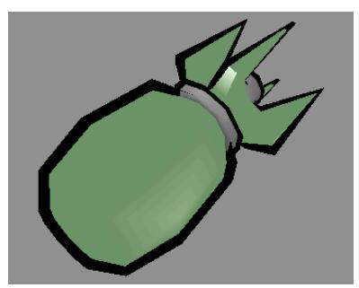
Figure 7-2: The black edges are actually a scaled version of the bomb, rendered with back-face culling, inverted normals, and no shading. Some artifacts are generated, but it generally gives pleasing results. (Image courtesy of ChrisEvans3D.com)
