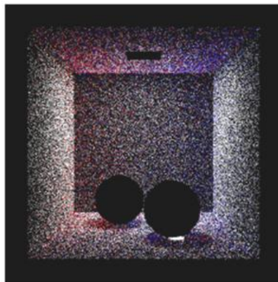
An example visualization of photons stored in the Photon Map. (Image taken from [Jensen00])
