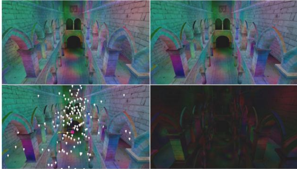
An example of injecting direct lights into a LPV. The white dots in the bottom left image are each individual point lights. By injecting them into the LPV, it is possible to fold massive amounts of direct lighting into the indirect lighting path. (Images from [Kaplanyan09])
