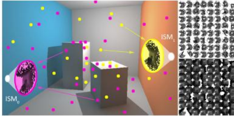
An example of Imperfect shadow maps. On the left, two ISMs are rendered, with the pink points representing geometry that gets rendered to ISM_0 and the yellow points being rendered to ISM_1 . On the right, we see two examples of 64 ISMs being stored in a large texture. The top set does not use the push/pull method of reconstruction, and the bottom one does. (Images taken from [RGKSDK08])
